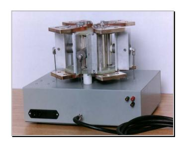
The Model 6025 is a two pole, three position pneumatically programmable reversing switch for use with the Model 6012M DCC Extender. The contacts are not designed to switch full current but are designed to carry the full current once switched. The switch is mounted 3" above the control box for easy accessibility to the lower contacts and is easily mounted within a 6-ft. standard equipment rack.
