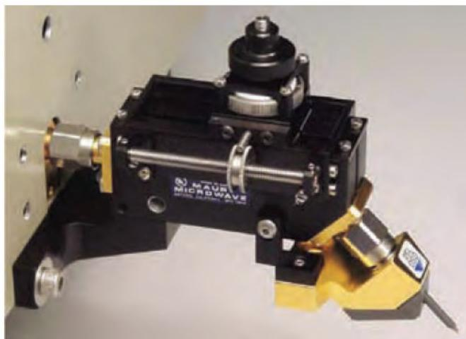
MT902A2 Pre-Matching Probe Mount on a MT989AU01 50 GHz Automated Tuner. This launch configuration is also used on MT902A1 and MT902A3.
